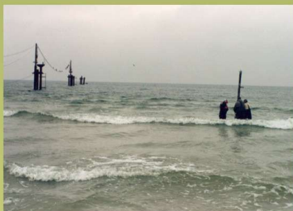
String wave gauge (manufactured at IBW PAN) + two-directional electromagnetic current meter (Valeport Ltd., UK) for measurements of waves and currents in shallow nearshore zone
