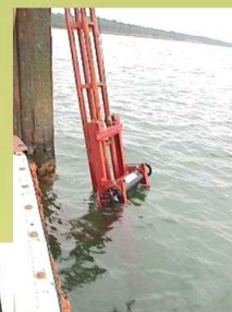
Particle Size Analyser LISST-100 for measurements of concentration and grain size distribution of suspended sediment (Sequoia Scientific, USA)
