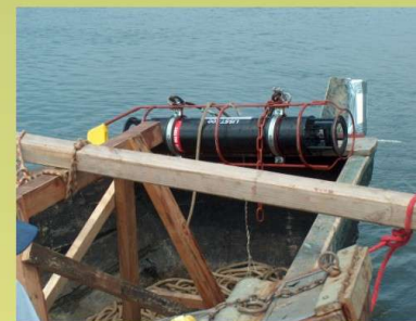
Particle Size Analyser LISST-100 for measurements of concentration and grain size distribution of suspended sediment (Sequoia Scientific, USA)
