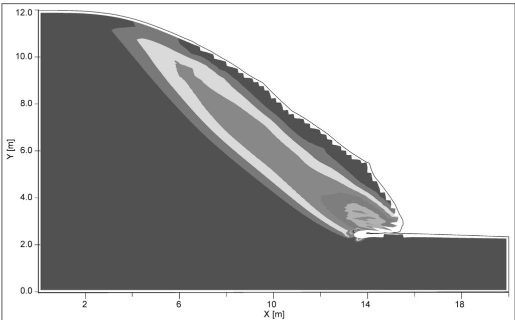
**Fig. 7.** Slide zone in the undercut dune
