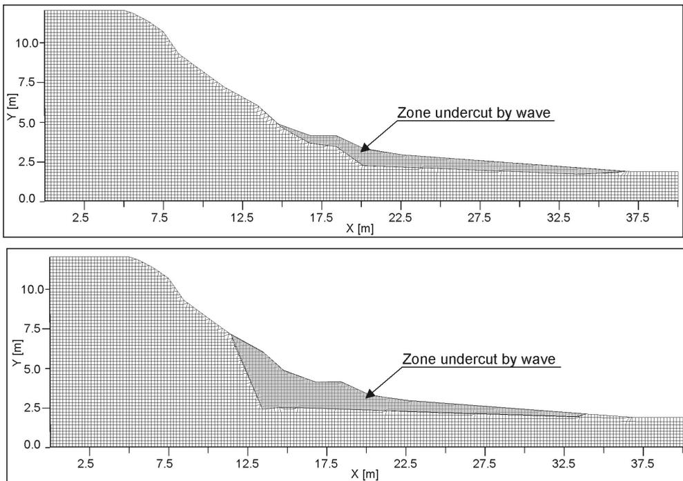
**Fig. 5.** Division of the dune model into finite difference zones:
