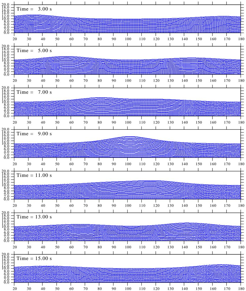
**Fig. 8.** Evolution of the discrete particle distribution during a collision of two solitary waves of the amplitudes  $A_1/H = 0.3$  and  $A_2/H = 0.2$ . The larger wave moves from the left to the right
