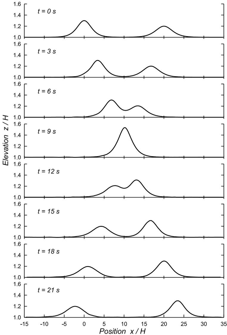
**Fig. 9.** Evolution of the free surface profiles of two colliding solitary waves of the amplitudes  $A_1/H = 0.3$  and  $A_2/H = 0.2$
