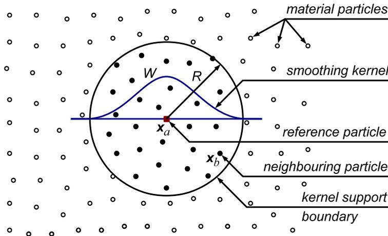
**Fig. 2.** Particle approximation involving material particles  $x_b$  (solid circles) located within a circular support domain of radius  $R$  around a reference particle  $x_a$  (solid square). Particles outside the support domain (empty circles) do not contribute to the approximation of field functions at  $x_a$ .  $W$  is the smoothing kernel function centred at  $x_a$ .
