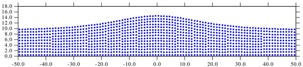
**Fig. 3.** Initial distribution of discrete particles. Labels along the axes show  $x$ - and  $z$ -coordinates in metres
