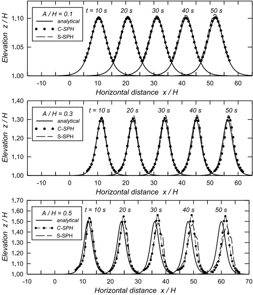
**Fig. 5.** Evolution of the water free surface for different dimensionless wave heights  $A/H$ , for the initial wave profile defined by the second-order solution of the KdV equation. Comparison of the corrected (C-SPH) and standard (S-SPH) results with analytical solutions
