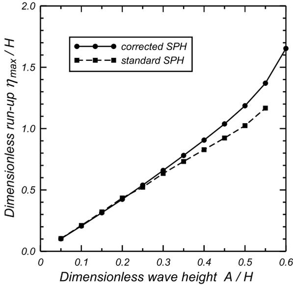
**Fig. 7.** Dependence of the maximum solitary wave run-up on the wave amplitude
