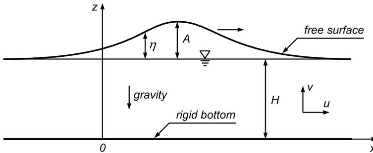
**Fig. 1.** Solitary wave problem definition: geometric parameters and coordinate axes
