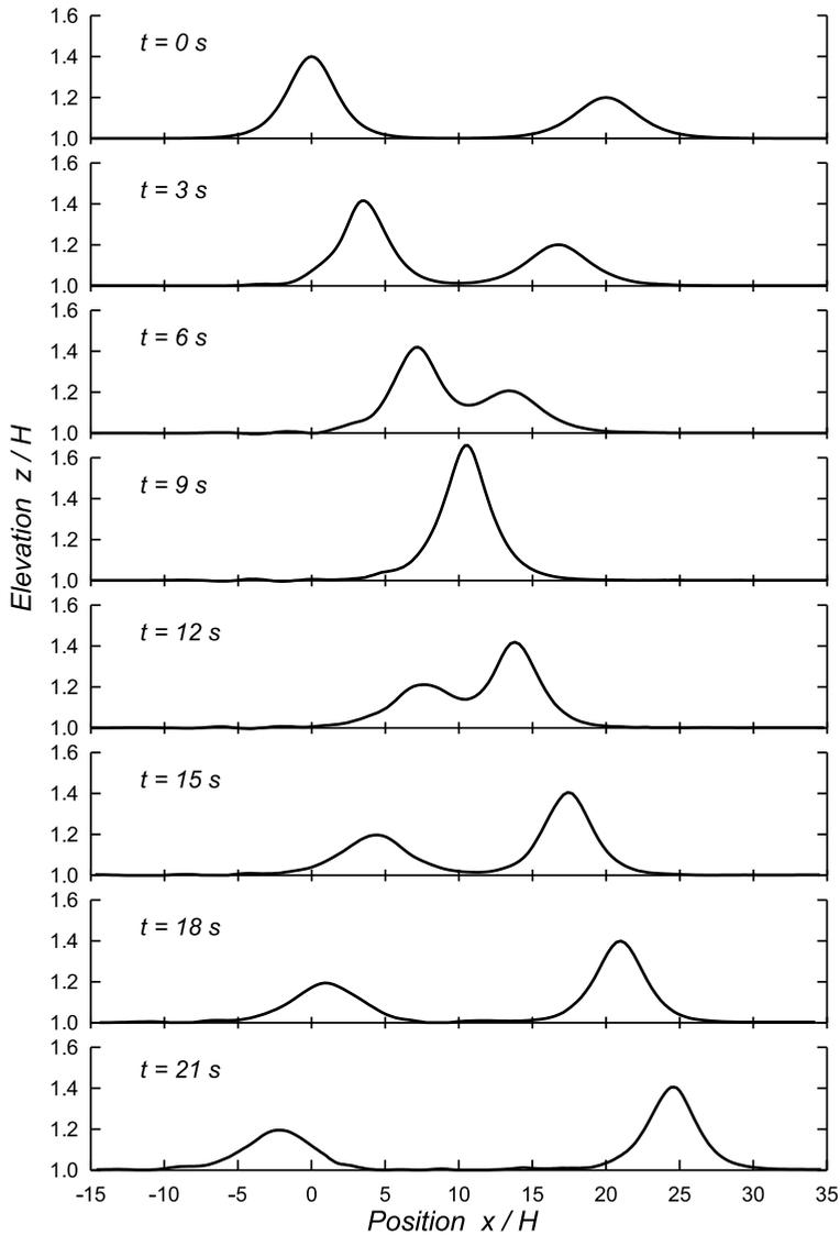
**Fig. 10.** Evolution of the free surface profiles of two colliding solitary waves of the amplitudes  $A_1/H = 0.4$  and  $A_2/H = 0.2$
