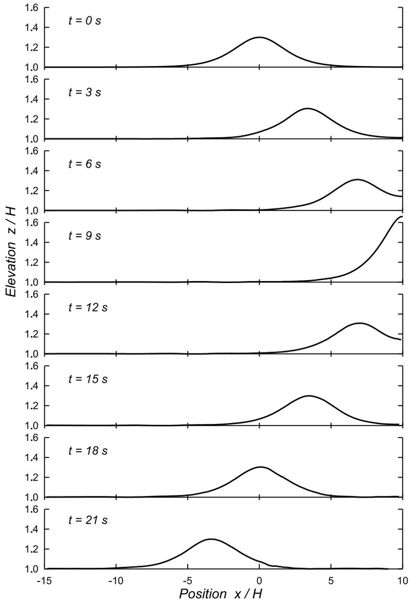
**Fig. 6.** Evolution of the free surface profile for a solitary wave of the amplitude  $A/H = 0.3$  impacting at a vertical wall at  $x/H = 10$
