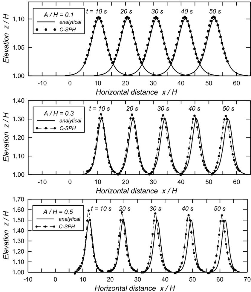
**Fig. 4.** Evolution of the water free surface for different dimensionless wave heights  $A/H$ , for the initial wave profile defined by the first-order solution of the KdV equation. Comparison of the numerical (C-SPH) results with analytical solutions
