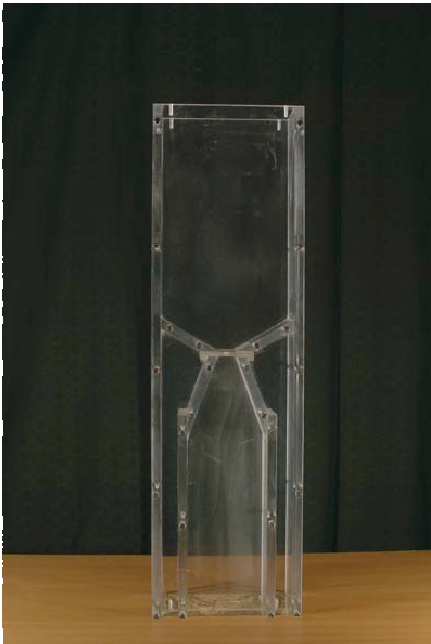
Fig. 8. Model silo with smooth walls: a) mass flow silo, b) funnel flow silo
