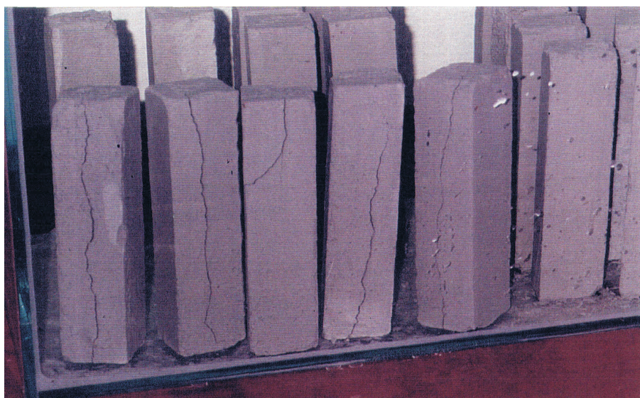
Photo 1. The samples of the slurry mixed with tap water (AW/R) after 69 days of storage in 1% solution of \text{Na}_2\text{SO}_4 , age of samples – 76 days
