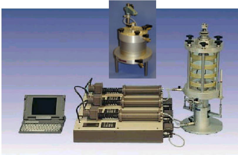
Fig 1. GDS Standard triaxial testing system, STDTTS showing optional Rowe and Barden consolidation cell (inset)
